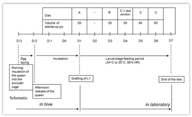
Figure 3 : Schematic representation of the important steps of the larval toxicity test (Source: OECD TG 237)
